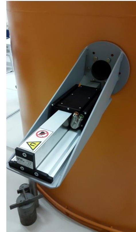
Linear motor drive during the second and third campaign
