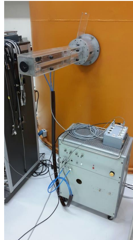
Pneumatic drive during the first campaign
