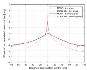
Fig. 2 Results for the homogeneous test case. All results were normalized to the same induced neutron noise in the fast energy group at the location of the noise source.
