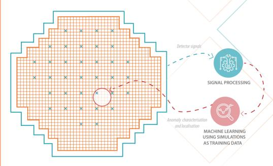
The project aims at first identifying regions of the core (conceptually highlighted in red) where a possible anomaly is located and at thereafter characterising the anomaly. The in-core instrumentation is represented by the crosses.
