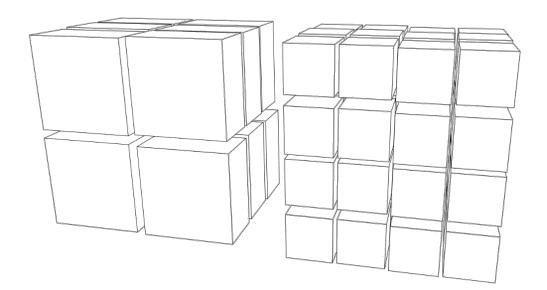
The initial 3D array of size 32 x 32 x 26 was compartmentalised into 12 and 48 subsections, by a factor 2 x 2 x 3 and 4 x 4 x 3 respectively.
